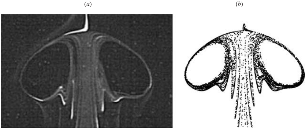
FIGURE 4. (a) Experiment with inclination \alpha = 0.4^\circ from Sotiropoulos et al. (2002). (b) Computation with inclination \alpha = 0.4^\circ , stretched 8 % vertically.
